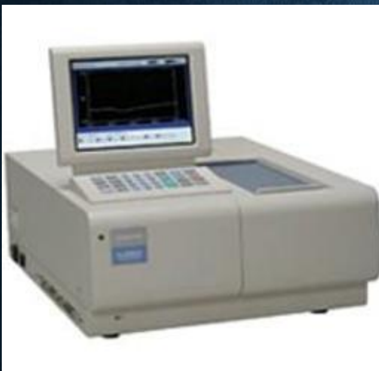
Hitachi U-2900 spectrophotometer
